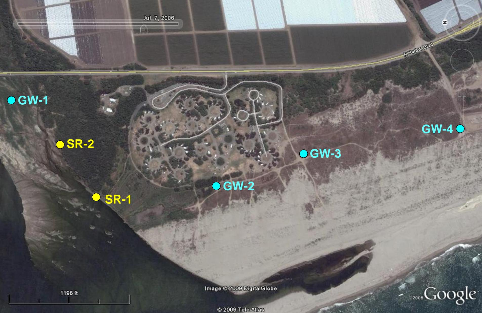
Figure 2-1 Proposed monitoring well (GW) and stage recorder (SR) locations (2006 aerial photograph)
